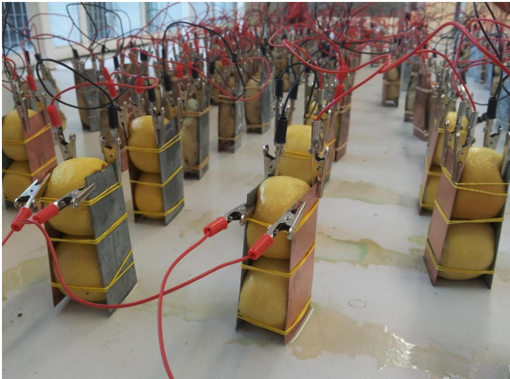
Lemon 'upgrade' to test for increased voltage and current
